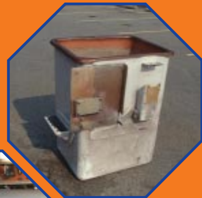
Fiberglass Utility Bucket Repairs
